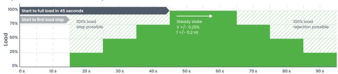
$Example\ profile\ for\ pre-heated/-lubricated;\ Without\ synchronization;\ 480\ V\ configuration;\ Power\ quality\ within\ +/-\ 10\%\ voltage,\ +/-5\%\ frequency$
